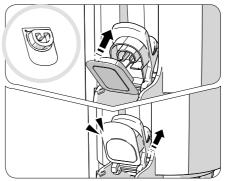
After cleaning, firmly insert with the round side outward and the grid hollow facing upward.
