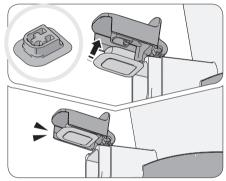
After cleaning, insert in a way that the round side of the packing faces outward while the grid grooves face upward.
