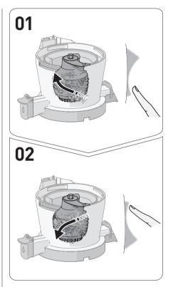
**01** For 2 to 3 times, repeat the process of pressing the operation switch in the **[REV]** direction for 3 to 5 seconds and then releasing it. The reverse rotation [REV] is a function that returns and lifts the ingredients upward. It only works when the switch is being pressed in the **[REV]** direction, and the screw rotation stops when the switch is released.
