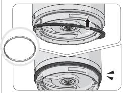
Assemble the packing as shown in the figure.
